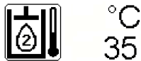
Fig.148387: Hydraulic oil temperature, hydraulic circuit 2 icon, display value and unit of measure
