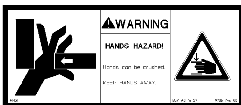
Fig.106030: Crushing danger for hands
