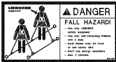
Fig.115119: Safety harness, maximum two persons
