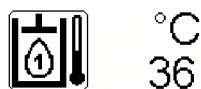
Fig.148386: Hydraulic oil temperature, hydraulic circuit 1 icon, display value and unit of measure
