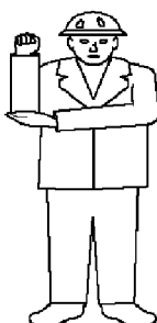
Fig.111720: Lifting with auxiliary winch
