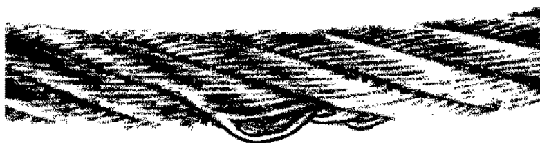
Fig.120991: Distorted or protruding strand
