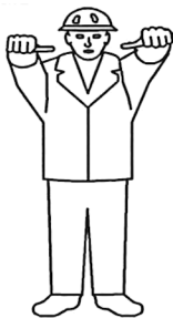
Fig.144250: Retracting the boom
