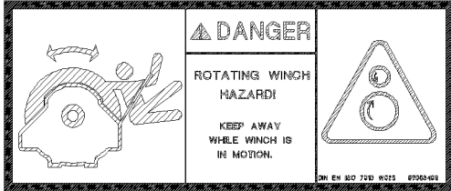
Fig.144738: Entanglement hazard during winch operation
