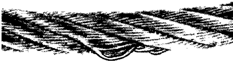
Fig.120991: Distorted or protruding strand
