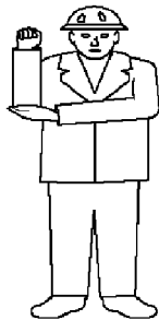
Fig.111720: Lifting with auxiliary winch
