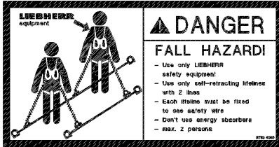
Fig.115119: Safety harness, maximum two persons
