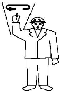
Fig.111706: Lift / lower a load with even speed
