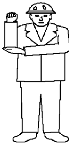
Fig.111720: Lift with auxiliary winch
