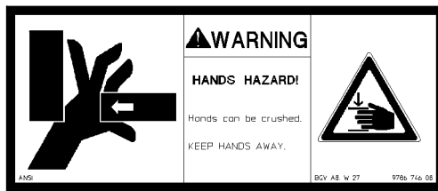
Fig.106030: Crushing danger for hands
