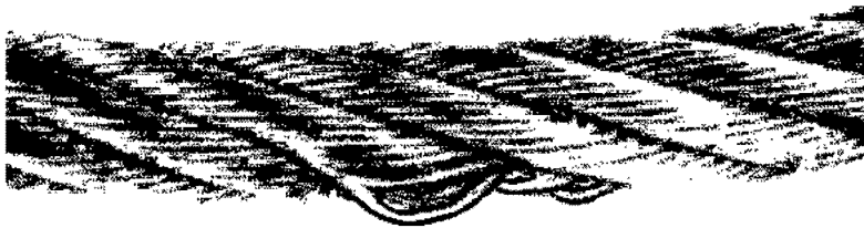
Fig.120991: Distorted or protruding strand
