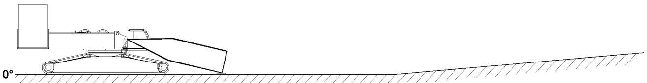
Fig. 121635: Boom - pivot section installed on turntable and placed on the ground
