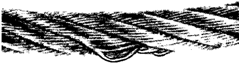
Fig.120991: Distorted or protruding strand
