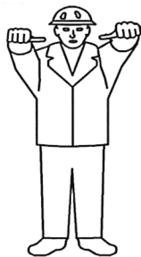
Fig.144250: Retracting the boom
