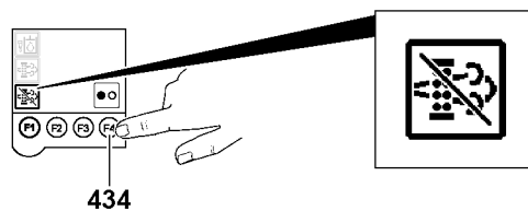
Fig.154109: Disabling automatic regeneration of the diesel particle filter
