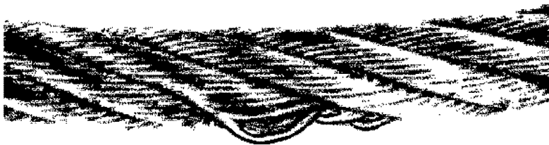
Fig.120991: Distorted or protruding strand
