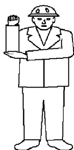
Fig.111720: Lifting with auxiliary winch
