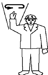
Fig.111706: Lifting / lowering a load with even speed
