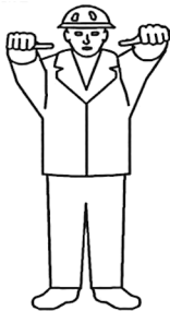
Fig.144250: Retracting the boom
