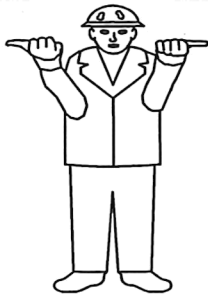
Fig.144249: Extending the boom
