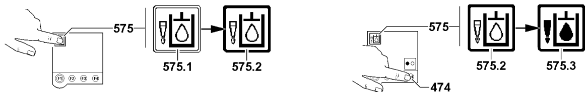
Fig.115320: Selecting the function Hydraulic oil preheating
