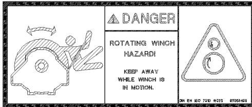
Fig.144738: Entanglement hazard during winch operation
