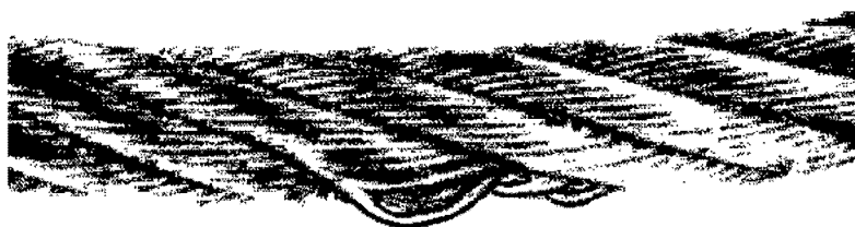
Fig.120991: Distorted or protruding strand
