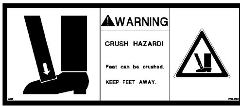
Fig.112474: Crushing danger for feet
