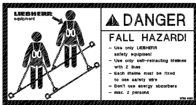
Fig.115119: Safety harness, maximum two persons
