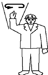
Fig.111706: Lifting / lowering a load with even speed
