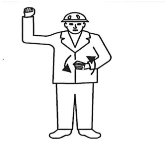
Fig.144248: Moving one crawler chain
