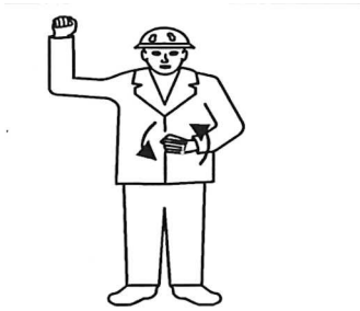
Fig.144248: Moving one crawler chain
