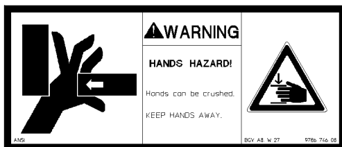
Fig.106030: Crushing danger for hands
