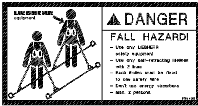
Fig.115119: Safety harness, maximum two persons
