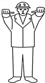
Fig.144250: Retracting the boom
