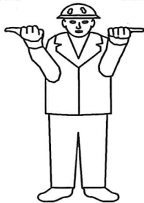
Fig.144249: Extending the boom
