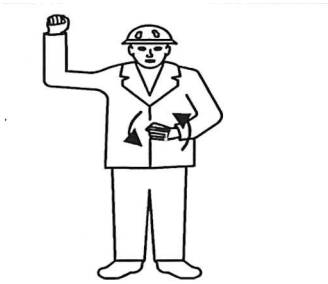
Fig.144248: Moving one crawler chain
