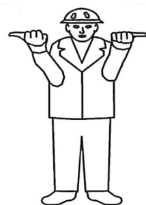
Fig.144249: Extending the boom
