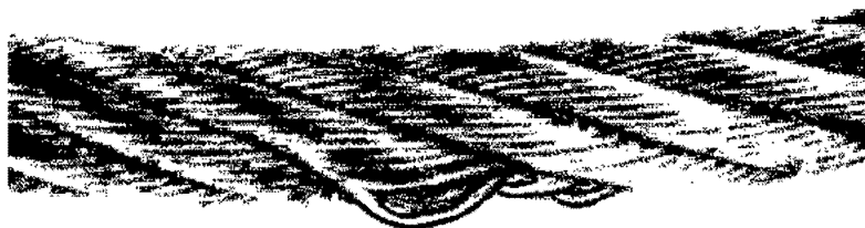
Fig.120991: Distorted or protruding strand
