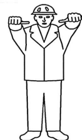
Fig.144250: Retracting the boom
