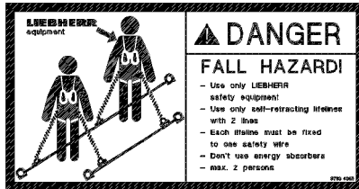
Fig.115119: Safety harness, maximum two persons
