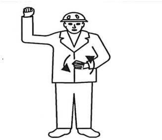
Fig.144248: Moving one crawler chain
