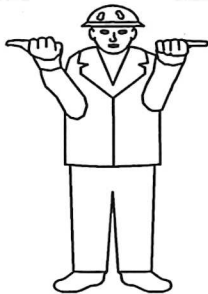
Fig.144249: Extending the boom
