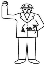
Fig.144248: Moving one crawler chain
