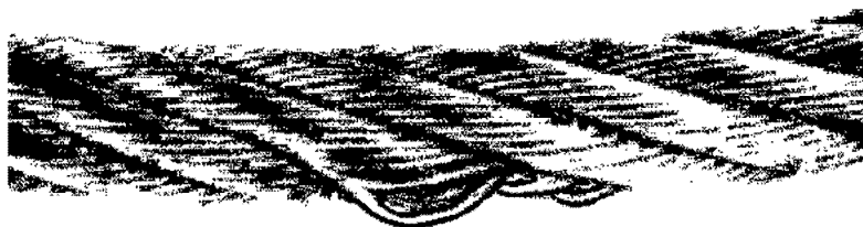
Fig.120991: Distorted or protruding strand
