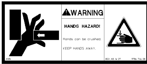
Fig.106030: Crushing danger for hands
