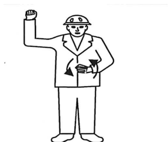
Fig.144248: Moving one crawler chain
