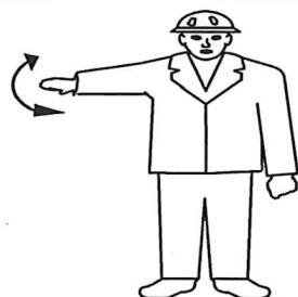
Fig.144245: Stop (normal stop)
