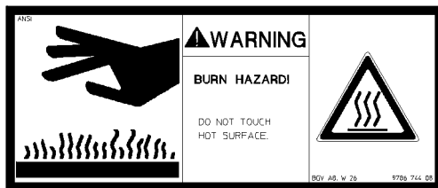
Fig.106028: Danger of burns to hands
