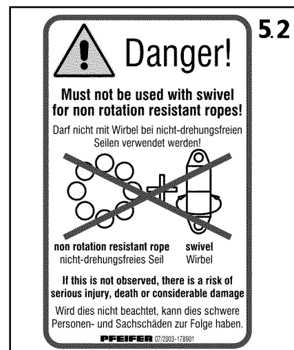
Fig.154084: Symbols for non-twisting ropes with rope end connections
