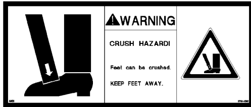
Fig.112474: Crushing danger for feet
