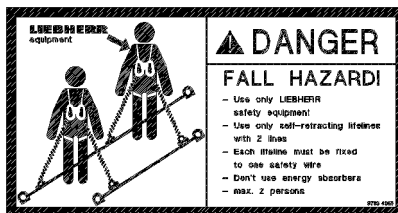
Fig.115119: Safety harness, maximum two persons
