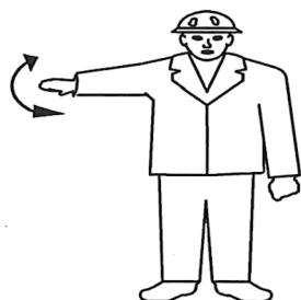
Fig.144245: Stop (normal stop)
