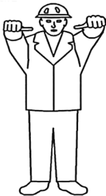
Fig.144250: Retracting the boom
