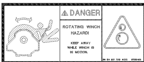
Fig.144738: Entanglement hazard during winch operation
