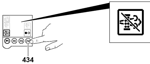
Fig.164442: Disabling automatic regeneration of the diesel particle filter
