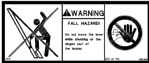
Fig.109032: Accessing the step ladder
