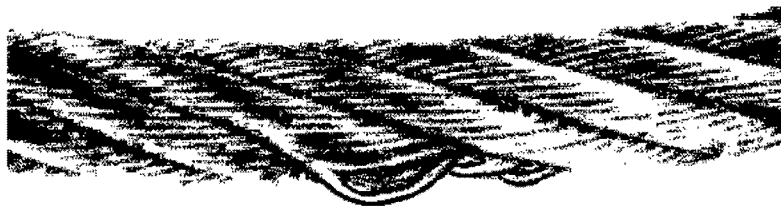
Fig.120991: Distorted or protruding strand
