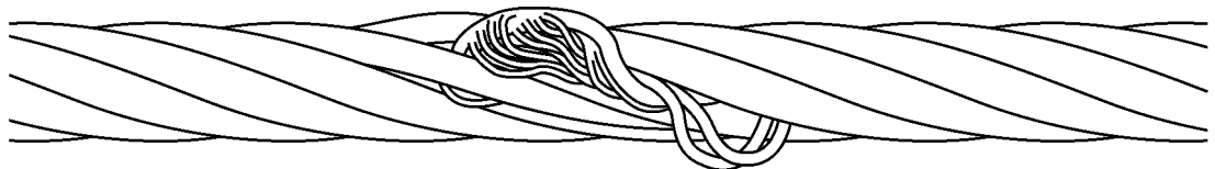
Fig.120990: Protrusion of an insert (rope single layer)
