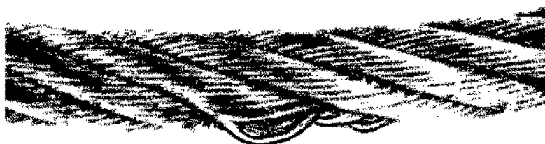
Fig.120991: Distorted or protruding strand
