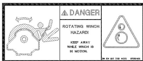
Fig.144738: Entanglement hazard during winch operation
