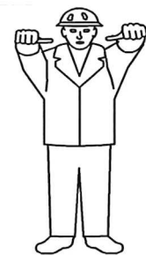
Fig.144250: Retracting the boom
