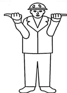
Fig.144249: Extending the boom
