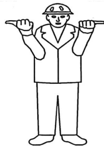
Fig.144249: Extending the boom
