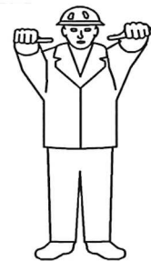
Fig.144250: Retracting the boom
