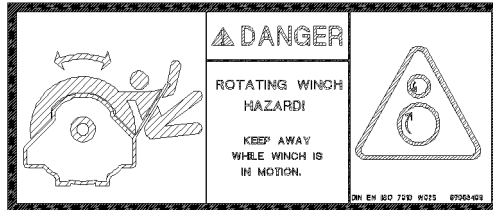
Fig.144738: Entanglement hazard during winch operation
