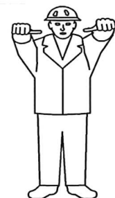
Fig.144250: Retracting the boom
