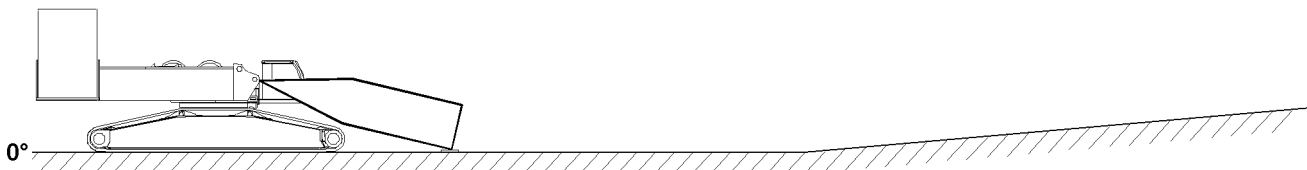
Fig.121635: Boom - pivot section installed on the turntable and taken down on the ground
