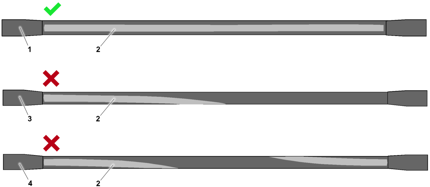
Fig.160904: Twisting marking for a straight fiber guy rope, example of a twisted fiber guy rope!
