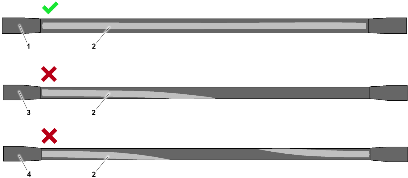
Fig.160904: Fiber guy rope, twisting marking for permissible alignment of the rope
