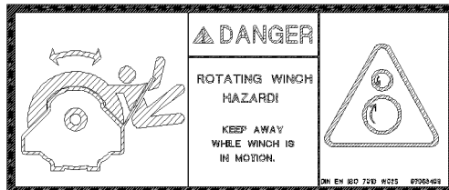
Fig.144738: Entanglement hazard during winch operation
