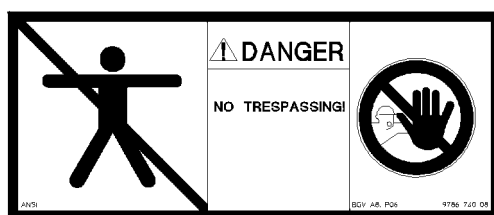
Fig.106037: Access for unauthorized personnel prohibited
