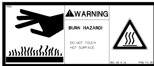
Fig.106028: Danger of burns to hands
