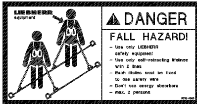
Fig.115119: Safety harness, maximum two persons
