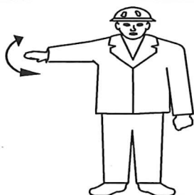
Fig.144245: Stop (normal stop)
