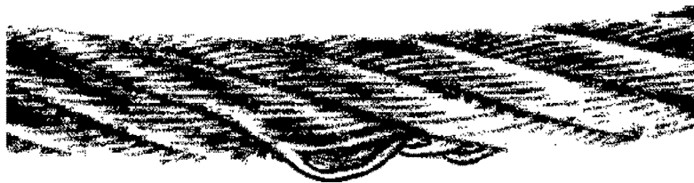
Fig.120991: Distorted or protruding strand
