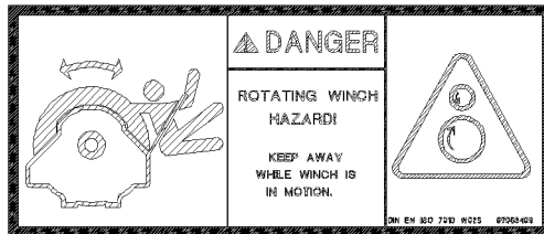
Fig.144738: Entanglement hazard during winch operation
