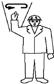
Fig.111706: Lifting / lowering a load with even speed
