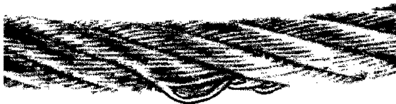
Fig.120991: Distorted or protruding strand
