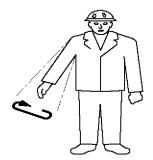
Fig.111708: Lower the load while stationary
