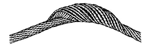
*Fig.120989: Basket formation* When basket formation is present, then the rope must be taken down.
