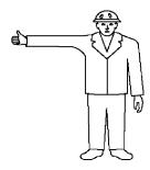
*Fig.111721: Lift the boom* Hold one arm horizontally with thumb directed upward.
