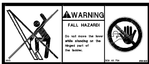
Fig.109032: Accessing the step ladder
