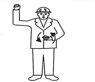
Fig.144248: Moving one crawler chain
