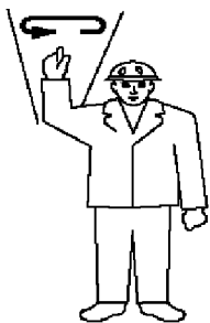
Fig.111706: Lifting / lowering a load with even speed
