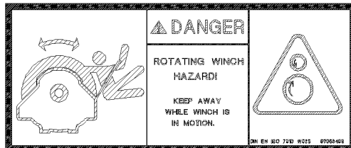
Fig.144738: Entanglement hazard during winch operation
