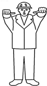
Fig.144250: Retracting the boom
