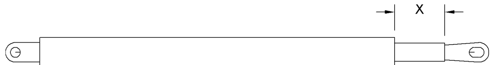
Fig. 5807: Minimum dimension x of the visible piston rod of the hydraulic tilting-back supports
