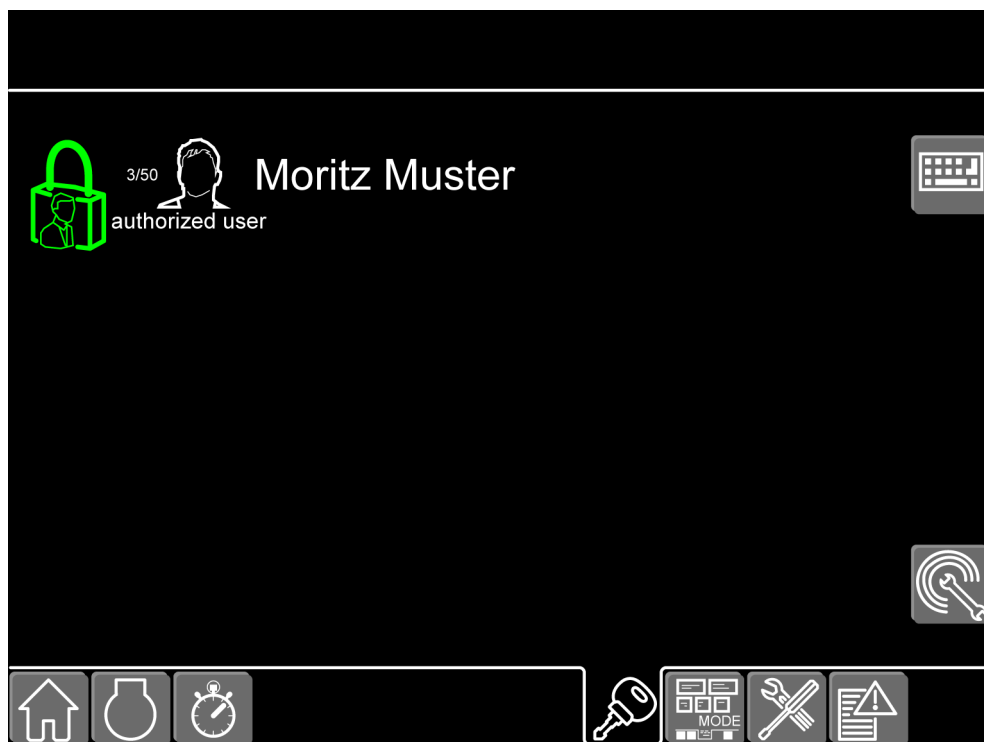
Fig. 1881: Access control screen - with retrofit kit access control (access with blue, user-specific ignition key)
