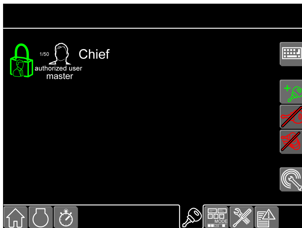
Fig. 1873: Screen Access control - with retrofit kit access control (access with red administrator ignition key)
