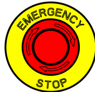
Fig. 2786: Emergency stop on control panel
