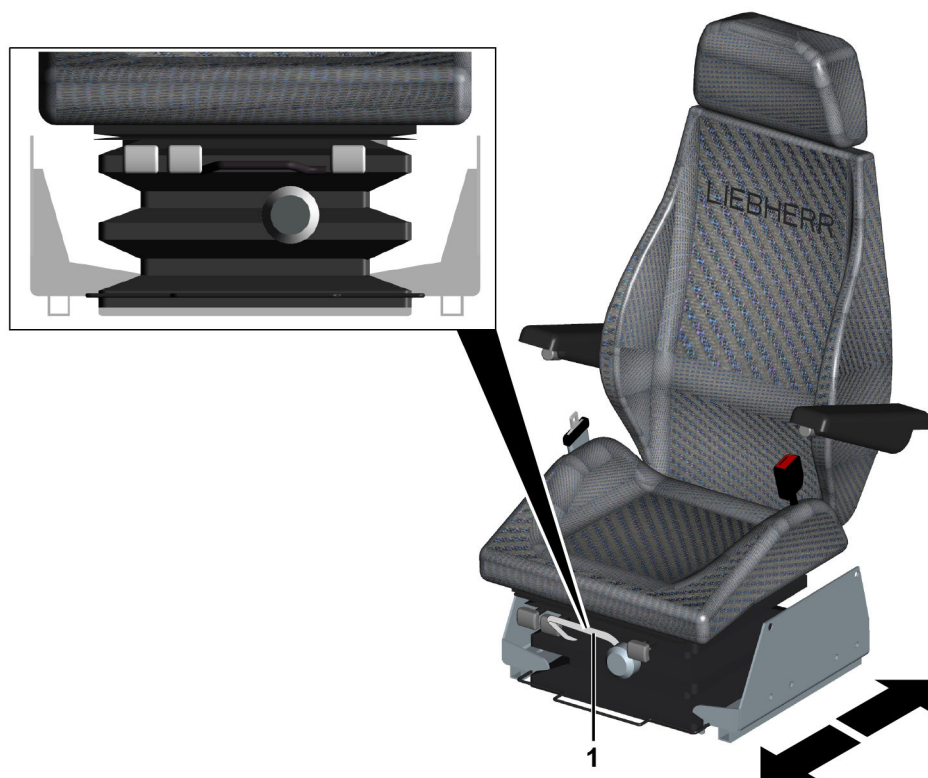
Fig. 2218: Adjusting the operator's seat horizontally
