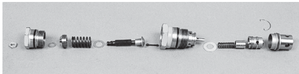
90000278 Multi-Function Valve Cartridge Components (Earlier production)
