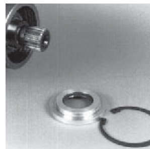
Fig. 50-10 - Seal Carrier Removed (Cartridge)
