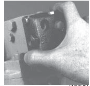
Fig. 50-43 - Remove HZ Control Housing
