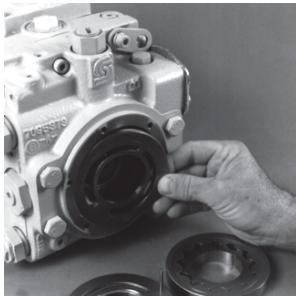
Install Inner Port Plate
