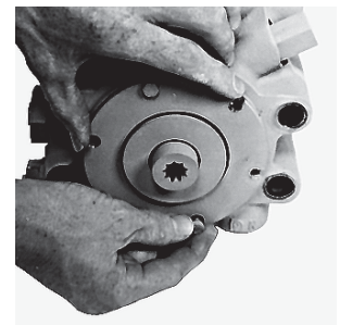
90000300 Install Screws and Cover Retainer
