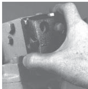
Fig. 50-47 - Install HZ Control Housing
