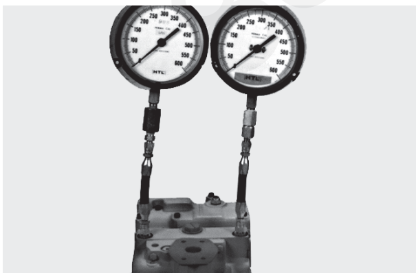
Install Gauges in Displacement Control Cylinder Gauge Ports
