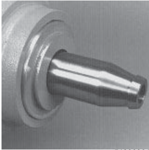
Fig. 50-12 - Install Seal Carrier (Cartridge)
