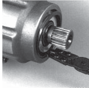
Fig. 50-13 - Install Carrier Retaining Ring (Cartridge)
