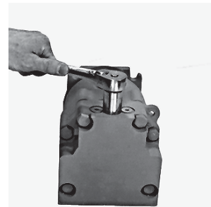
90000342 Remove Shim Charge Relief Valve
