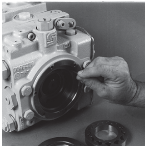
Install Alignment Pin
