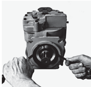
90000271 Remove Seal Carrier
