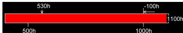
Fig. 1583: Maintenance intervals - maintenance interval past due (lit red)
