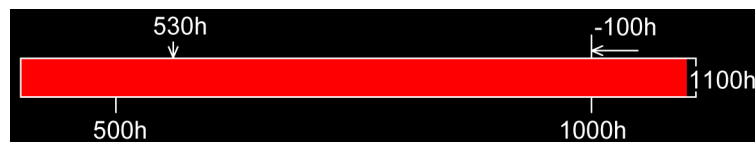
Fig. 1562: Maintenance intervals - maintenance interval past due (lit red)
