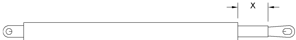
Fig. 5773: Minimum dimension x of the visible piston rod of the hydraulic tilting-back supports
