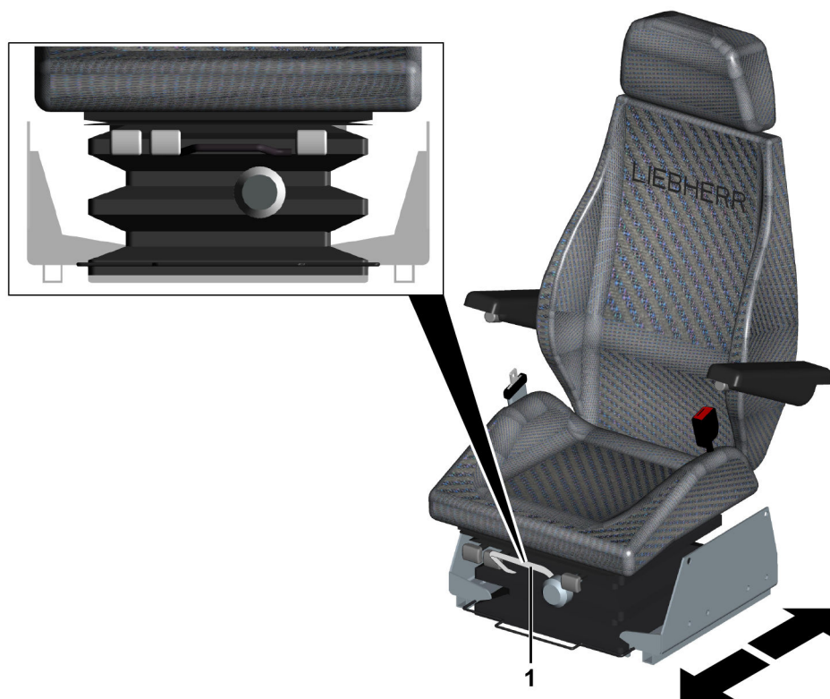
Fig. 2218: Adjusting the operator's seat horizontally
