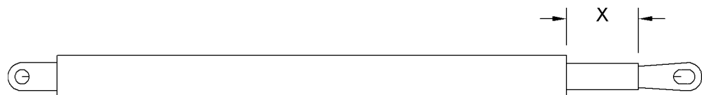
Fig. 5362: Minimum dimension x of the visible piston rod of the hydraulic tilting-back supports
