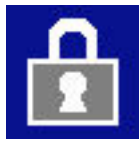
Fig. 2688: Symbol Radio remote control blocked (blinks)
