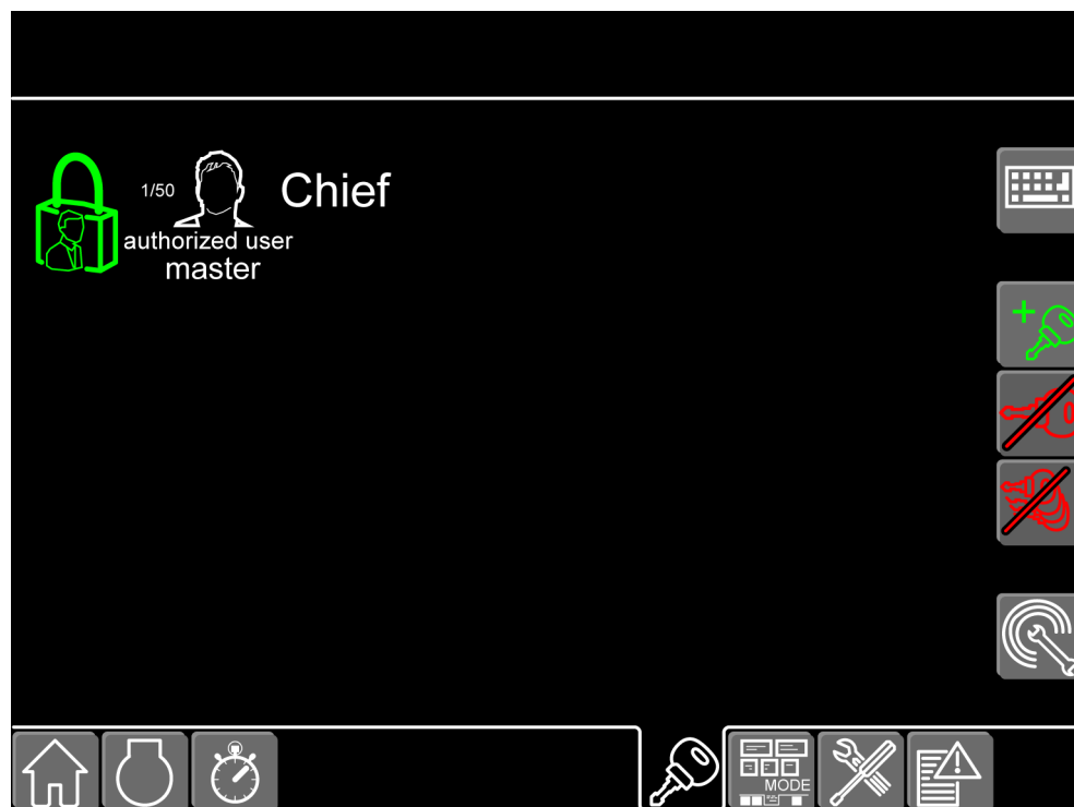
Fig. 1892: Screen Access control - with retrofit kit access control (access with red administrator ignition key)
