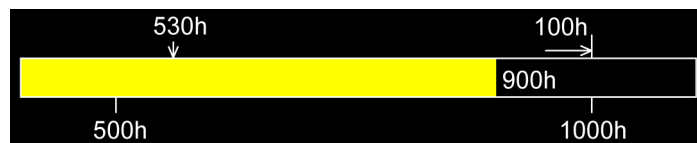
Fig. 1582: Maintenance intervals - maintenance intervals pending shortly (lit yellow)
