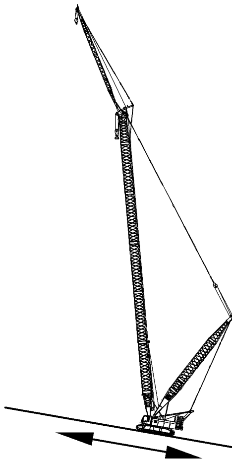
Fig. 2898: Permitted gradient for main boom 2821 + fixed jib 0906 + derrick, boom travel uphill
