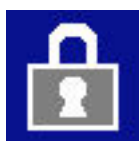
Fig. 2663: Symbol Radio remote control blocked (blinks)
