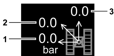
Fig. 2684: Screen clipping Ground pressure
