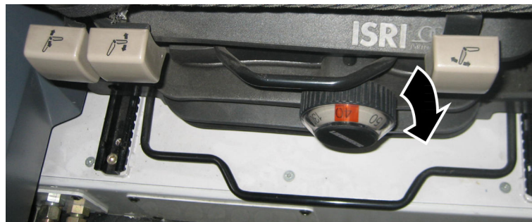
Fig. 2223: Decreasing the dampening
