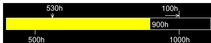
Fig. 1563: Maintenance intervals - maintenance intervals pending shortly (lit yellow)
