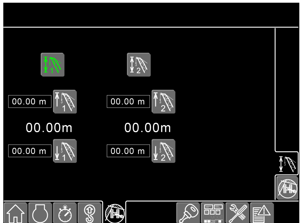
Fig. 1853: Screen Working range limitation - lifting height limitation
