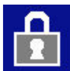
Fig. 2658: Symbol Radio remote control blocked (blinks)
