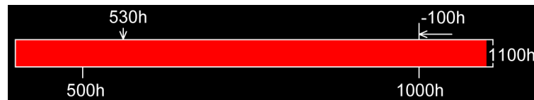
Fig. 1564: Maintenance intervals - maintenance interval past due (lit red)
