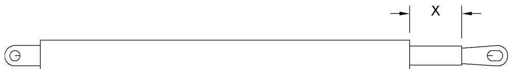
Fig. 5289: Minimum dimension x of the visible piston rod of the hydraulic tilting-back supports
