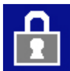
Fig. 2656: Symbol Radio remote control blocked (blinks)
