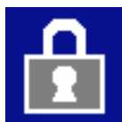
Fig. 2661: Symbol Radio remote control blocked (blinks)
