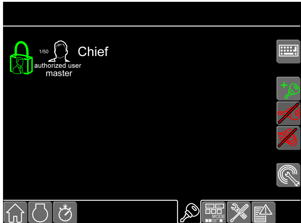
Fig. 1871: Screen Access control - with retrofit kit access control (access with red administrator ignition key)
