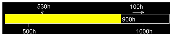
Fig. 1561: Maintenance intervals - maintenance intervals pending shortly (lit yellow)
