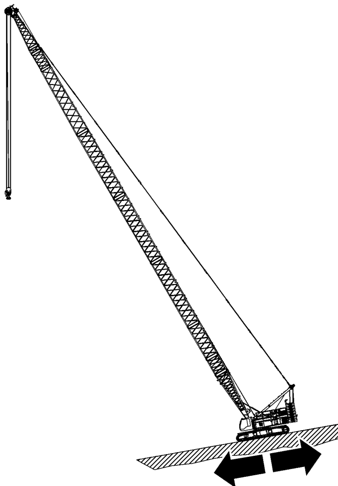
Fig. 2845: Permitted gradient for main boom 2821 + reducing adapter 2821/2316, boom travel downhill
