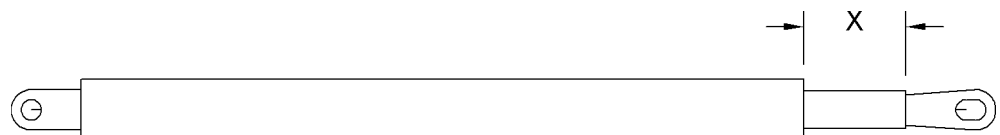
Fig. 2928 Minimum dimension x of the visible piston rod of the hydraulic tilting-back supports
